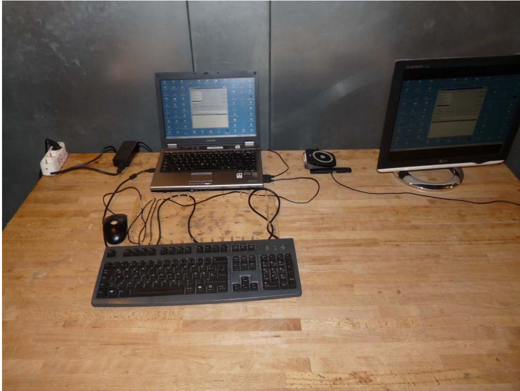
Photo 6: Test setup for conducted measurements (computer peripheral setup, EUT supplied by USB-cable from computer, unintentional radiator §15)
