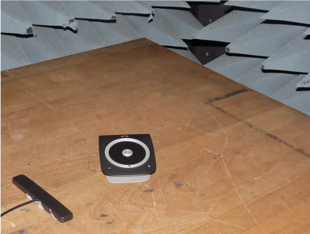
Photo 1: Test setup for radiated measurements (Enclosure, below 30 MHz, intentional radiator §15)
