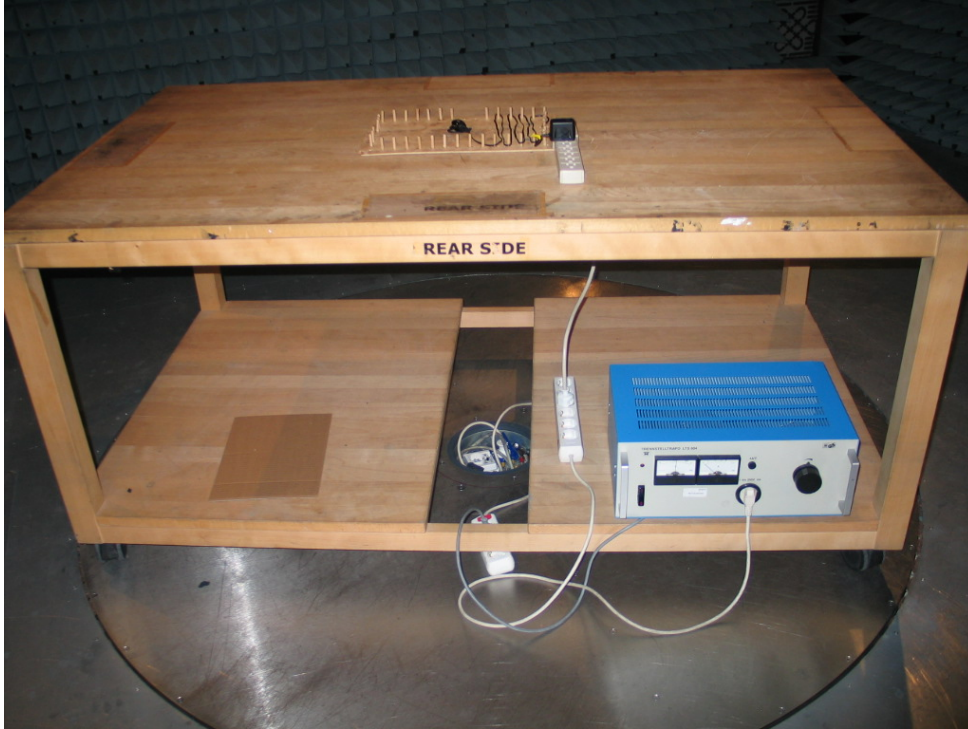
Photo 1: Test setup for radiated measurements (with charger)
