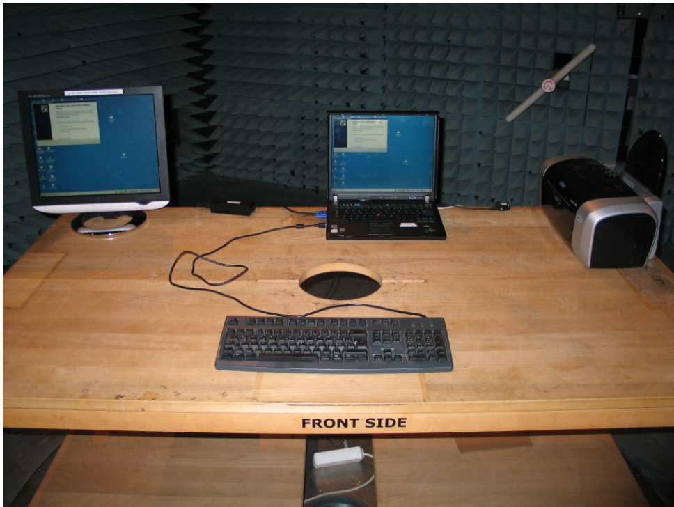
Photo 2: Test setup for radiated measurements (with Computer periphery)
