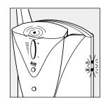
7. Put the System in Headset Mode. The Headset Mode light on the top of the Remote blinks, and the Headset Mode light on the side of the Base illuminates. It will take up to 45 seconds to establish a channel with first use.
