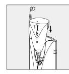
6. Slide the Remote into the Charger on either side of the Base. The Battery Charge light on the side of the Base illuminates. Charge the Battery for a full 3 hours. Use the Handset while the Battery charges.
