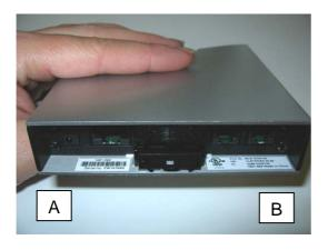
Place one of the serial no labels on the inside Buttom of the base (A), and place the approval Label In same area (B)
