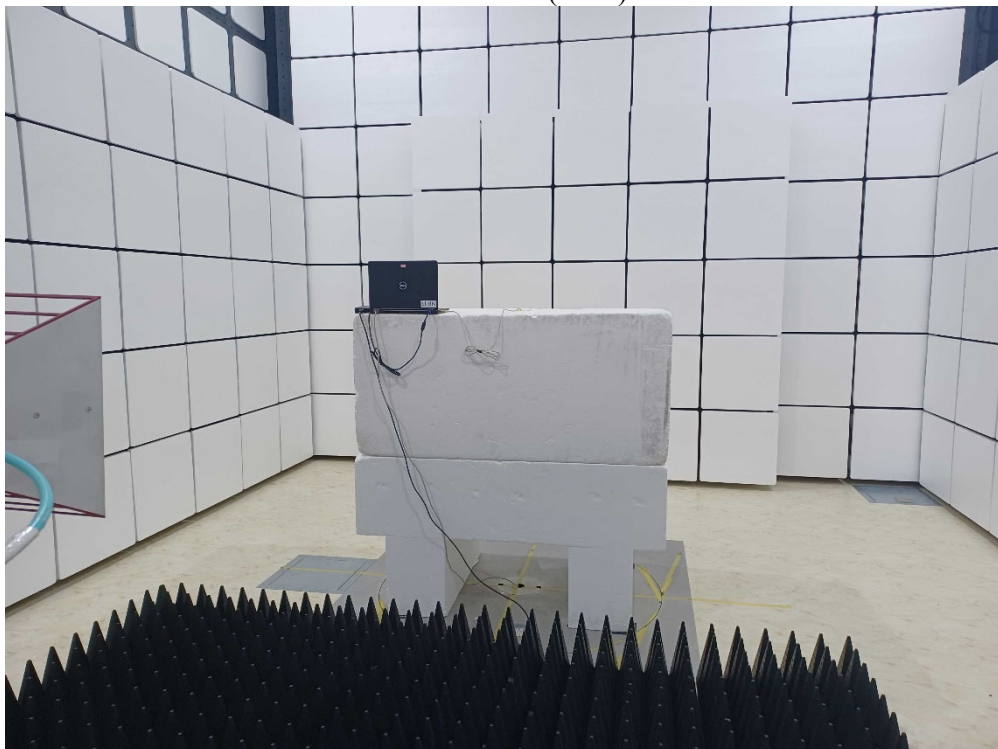
Radiated Test (Horn)
