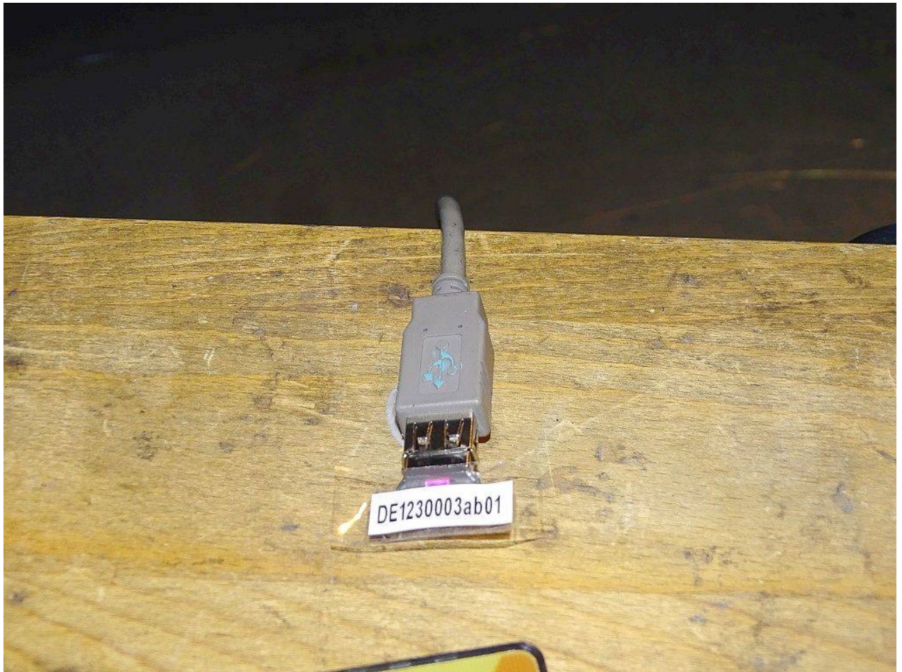
Photo 6: Detail of EUT setup for radiated measurements (computer peripheral setup, EUT supplied by USB-cable from computer, unintentional radiator §15.109, ANSI C63.4) Frequency Range: 30 MHz – 1 GHz
