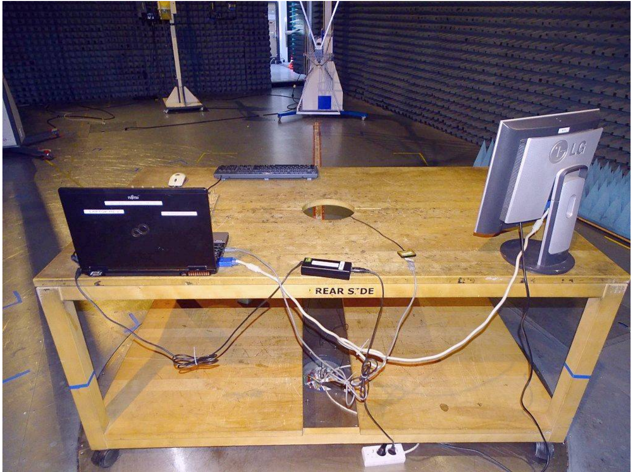
Photo 7: Test setup for radiated measurements (computer peripheral setup, EUT supplied by USB-cable from computer, unintentional radiator §15.109, ANSI C63.4) Frequency Range: 30 MHz – 1 GHz
