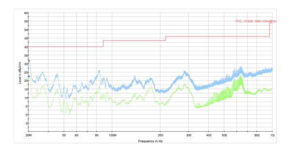
AC mains connection = via connected computer device, Measurement range = 30 MHz - 1 GHz, Test setup = computer peripheric
