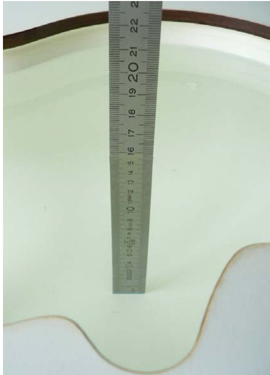
Fig. 16: Liquid depth for 2450 MHz Head measurements.
