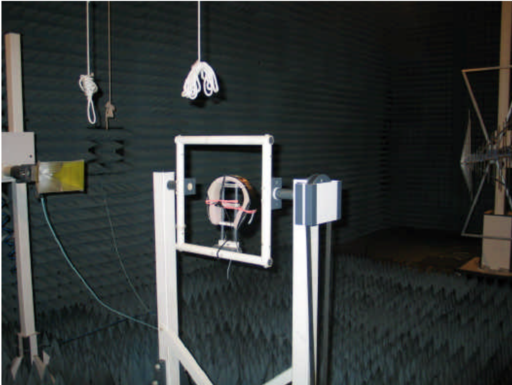
Photo 1: Test setup for radiated measurements (above 1 GHz)
