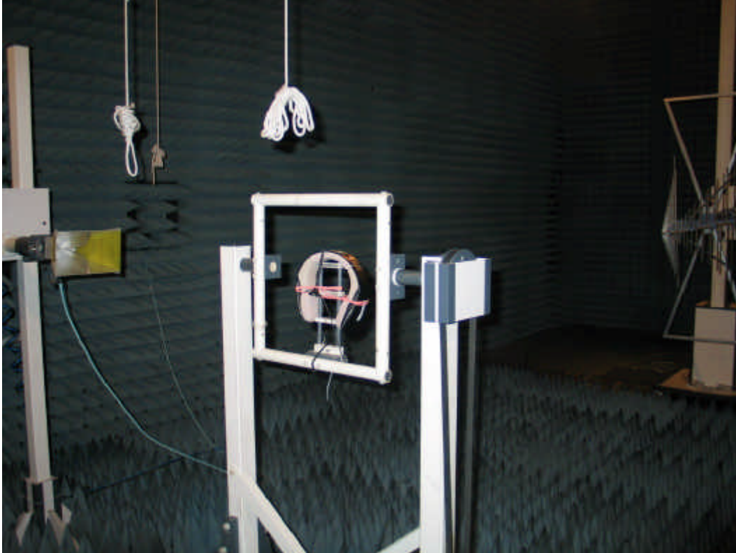
Photo 1: Test setup for radiated measurements (above 1 GHz)
