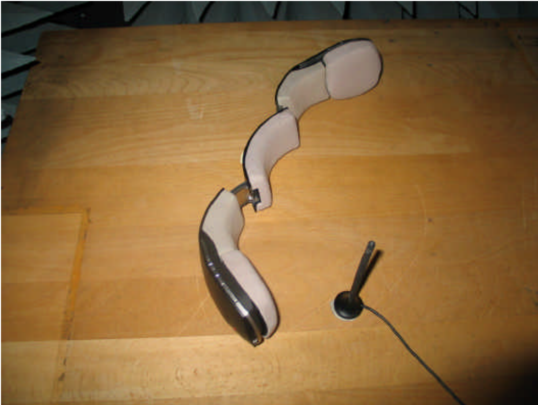
Photo 3: Test setup for radiated measurements (below 30 MHz)
