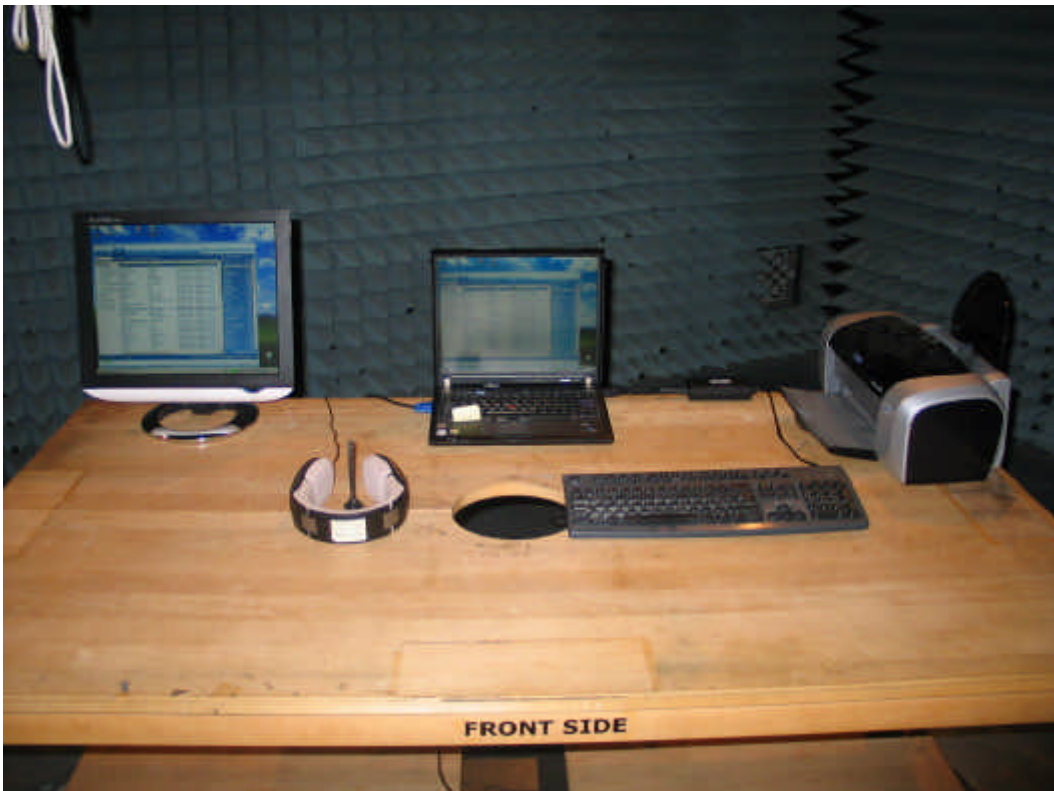
Photo 2: Test setup for radiated measurements (30 MHz up to 1 GHz)
