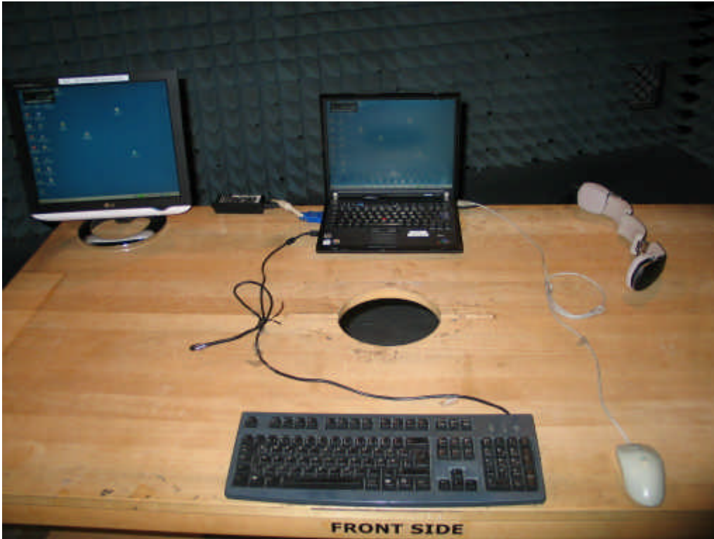
Photo 1: Test setup for radiated measurements
