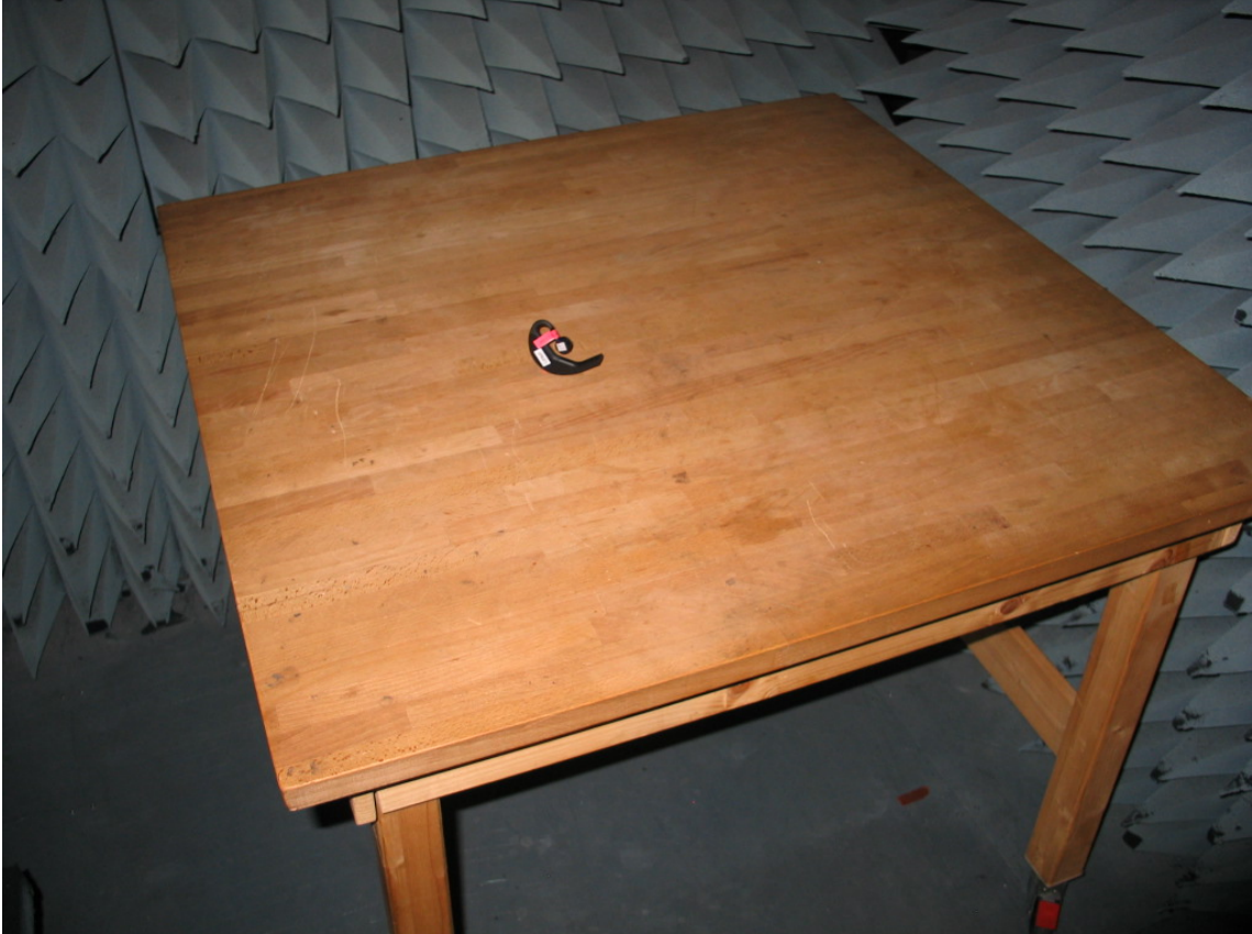
Photo 1: Test setup for radiated measurements (below 30 MHz)
