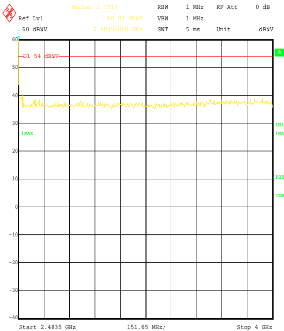
Title: GN Netcom EUT: BT 135 FCC Part 15.247. Rad Emissions Comment A: 48063JD05 TX Mode. Top Channel Date: 18.APR.2006 19:32:38
