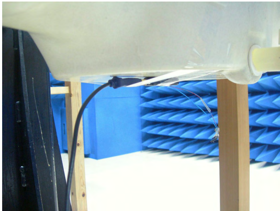
Figure 11. Body SAR Test Setup (Flat Section)
