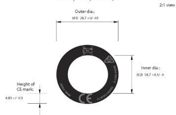
Facestock: Polyester Rear side adhesive: Acrylic, permanent, to fit ABS plastic parts Dimensions: As shown above Thickness: 0.1 mm +/-0.05 Supply form: On roll for. Labels on outer side on roll
