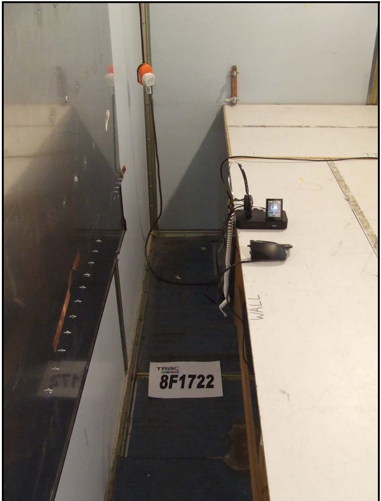
PHOTOGRAPH No. 2 POWERLINE CONDUCTION TEST SETUP
