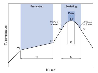
Soldering Preheating Critical zone (T3 to T4) Peak Temp. Time Temp. Time Temp. Time T1 T2 **T**4 t1 Т3 t2 t3\* 150°C 200°C 60 to 120sec 217°C 60 to 120sec 240 to 260°C 30sec max.
