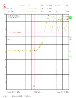
Transmitter Band Edge Radiated Emissions: Section 15.247(c) & 15.209(a) (Continued)
