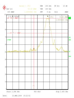
Transmitter Band Edge Radiated Emissions: Section 15.247(c) & 15.209(a) (Continued)
