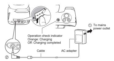
When disconnecting the adapter from the camera, always disconnect the camera end of the cable (② in the above diagram) first.
