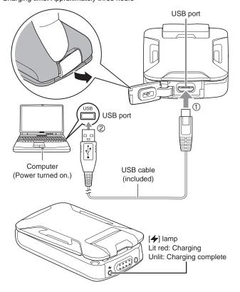
• Charging from a non-computer device's USB port You can charge the sensor unit from a USB port (Type-A) that complies with USB standards.
