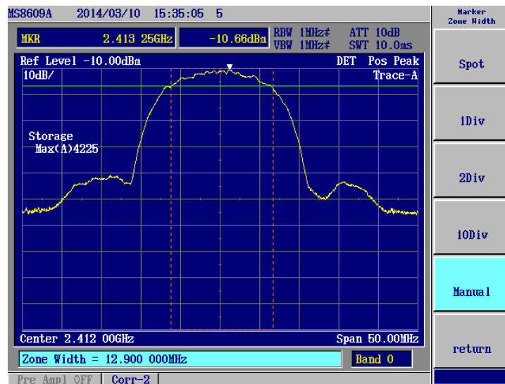
Figure 1 6dB Bandwidth(Lower ch_2412.000MHz)
