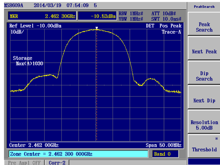
Figure 6 Maximum Peak Output Power(Higher ch_2462.000MHz)
