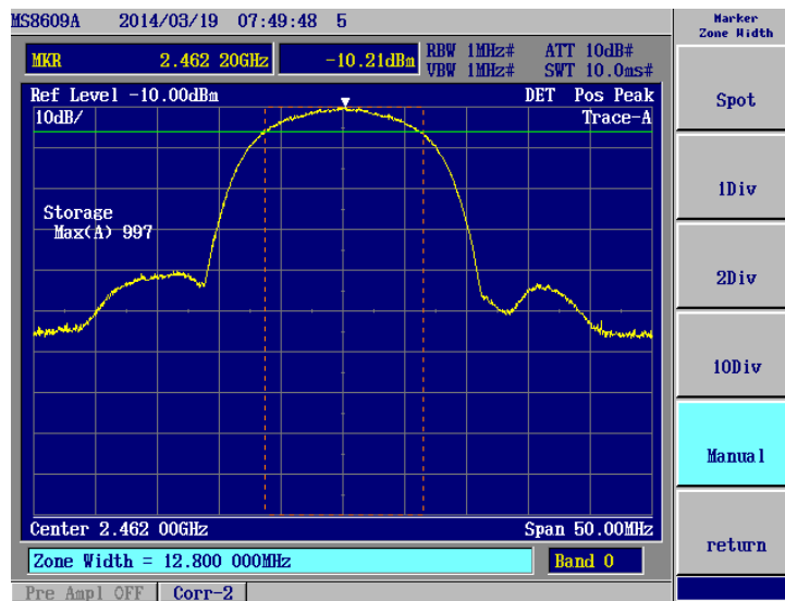
Figure 3 6dB Bandwidth(Higher ch_2462.000MHz)
