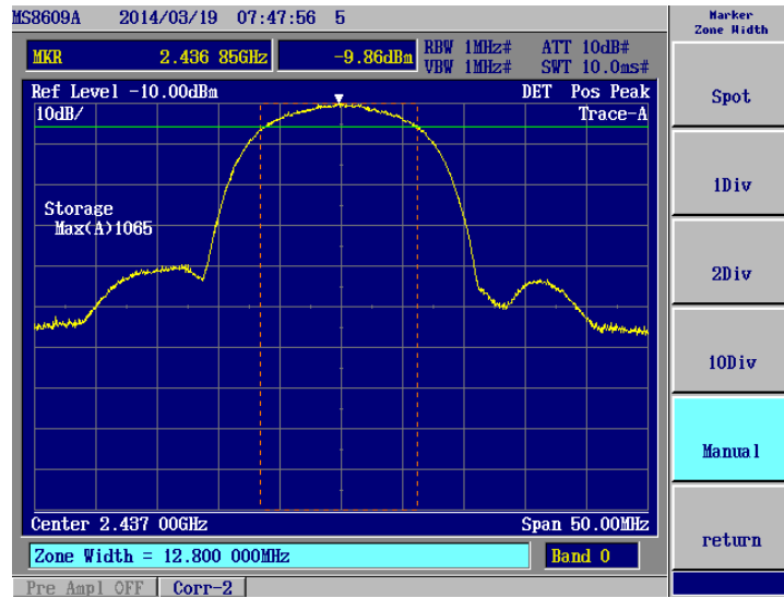
Figure 2 6dB Bandwidth(Middle ch_2437.000MHz)
