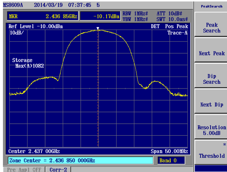
Figure 5 Maximum Peak Output Power(Middle ch_2437.000MHz)
