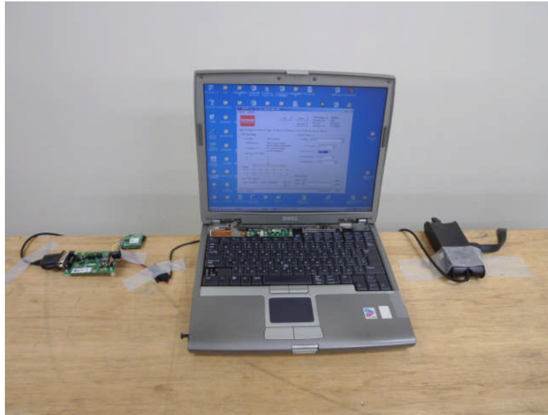
Photo5 Test setup for Line conducted(Front)
