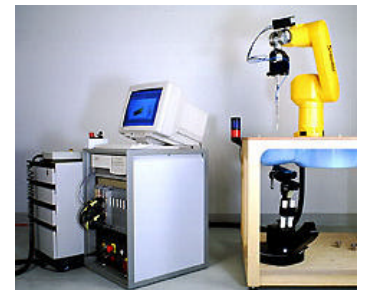
Fig. 1 SAR Test Setup
