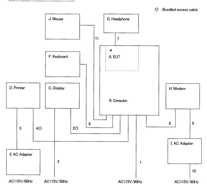
Symbols or numbers assigned to equipment or cables on this diagram are corresponded to the symbols or numbers assigned to equipment or cables on tables in Configuration/Cable Information.
