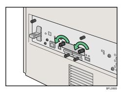
The removed cover is not used when installing the interface board.
