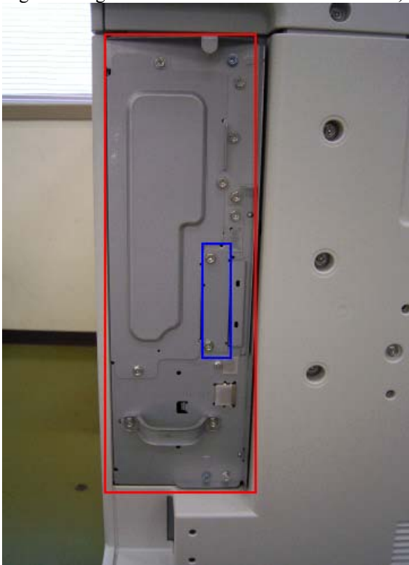
Fig 2. Enlarged view of Location of “R-WL54MG, R-WL54CG” to be equipped for a printer (example)
