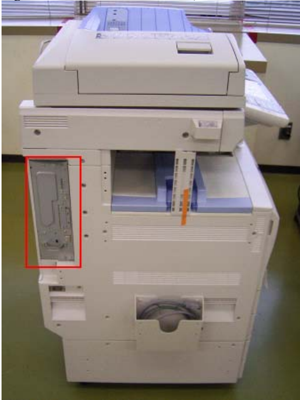
Fig 2. Enlarged view of Location of “R-WL54MG, R-WL54CG” to be equipped for a printer (example)
