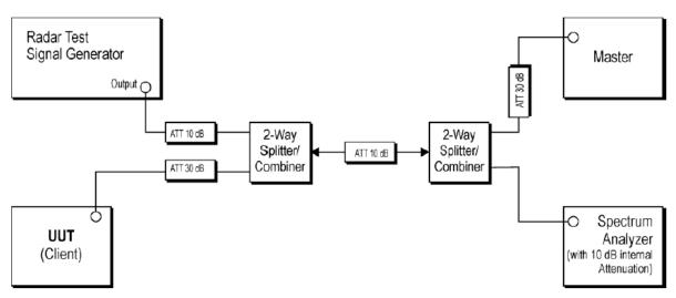
Radar Test Waveforms are injected into the Master.
