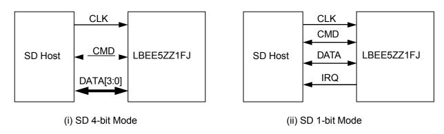
Note : 10 to  $100k\Omega$  pull-ups are required on the four DATA lines and the CMD line. This requirement must be met during all operating states by using external pull-up resisters or properly programming internal SDIO host pull-ups.
