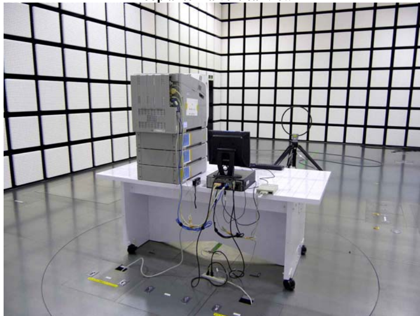
Loop antenna vertical view
