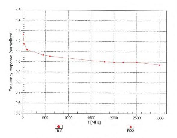
Frequency Response of E-Field (TEM-Cell:ifi110 EXX, Waveguide: R22)
