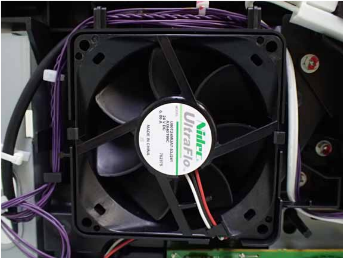
Figure 27 Internal View (DC Fan #1)
