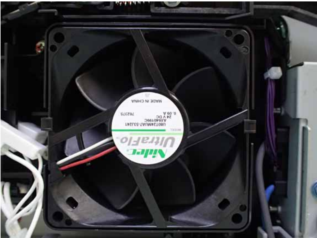
Figure 28 Internal View (DC Fan #2)
