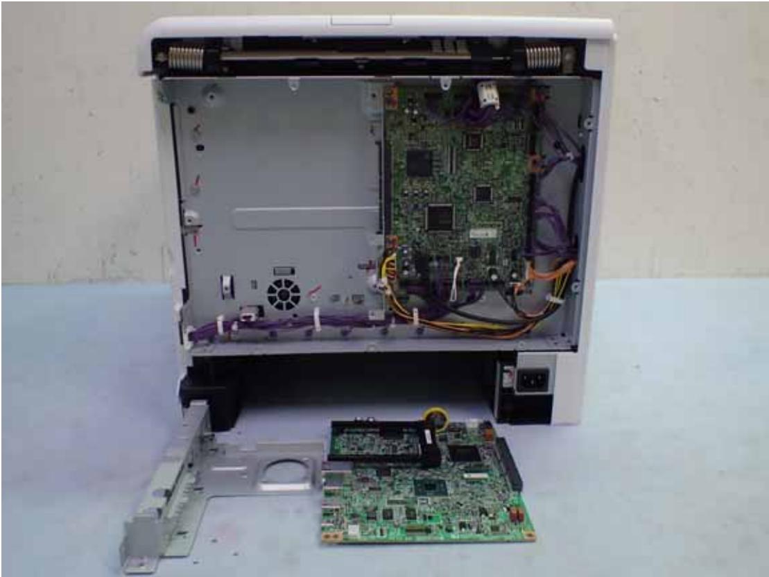
Figure 23 Internal View (Removed Main Board #2)
