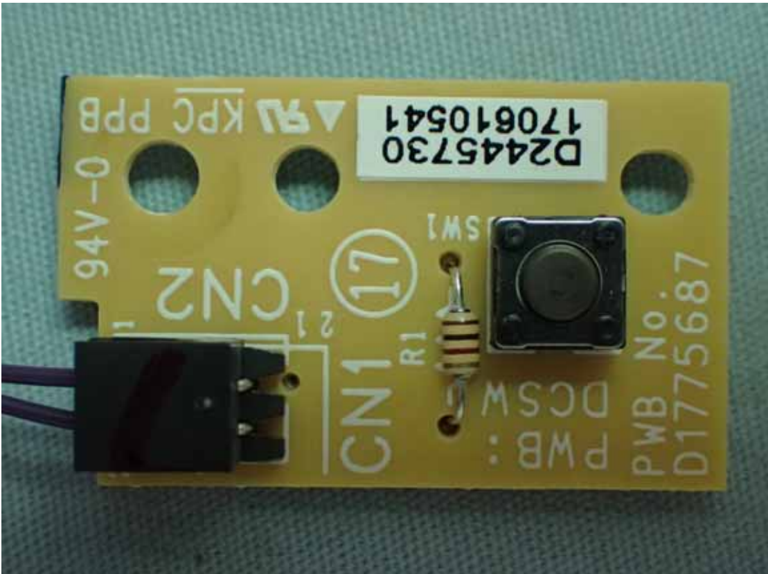
Figure 36 Internal View (SW Board, Front View)
