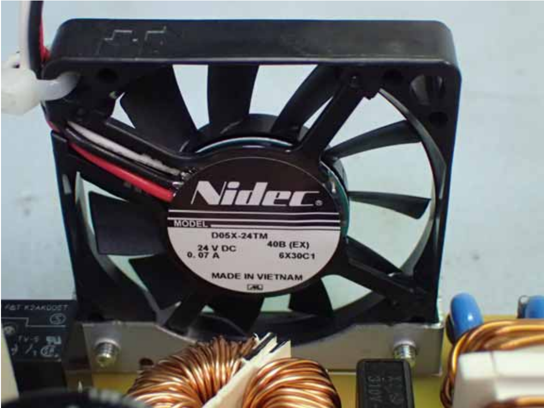
Figure 35 Internal View (DC Fan of Power Board)
