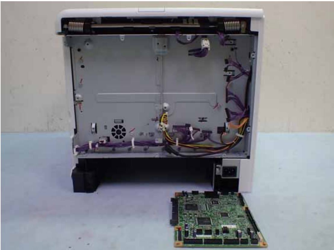
Figure 20 Internal View (Removed Main Board #1)
