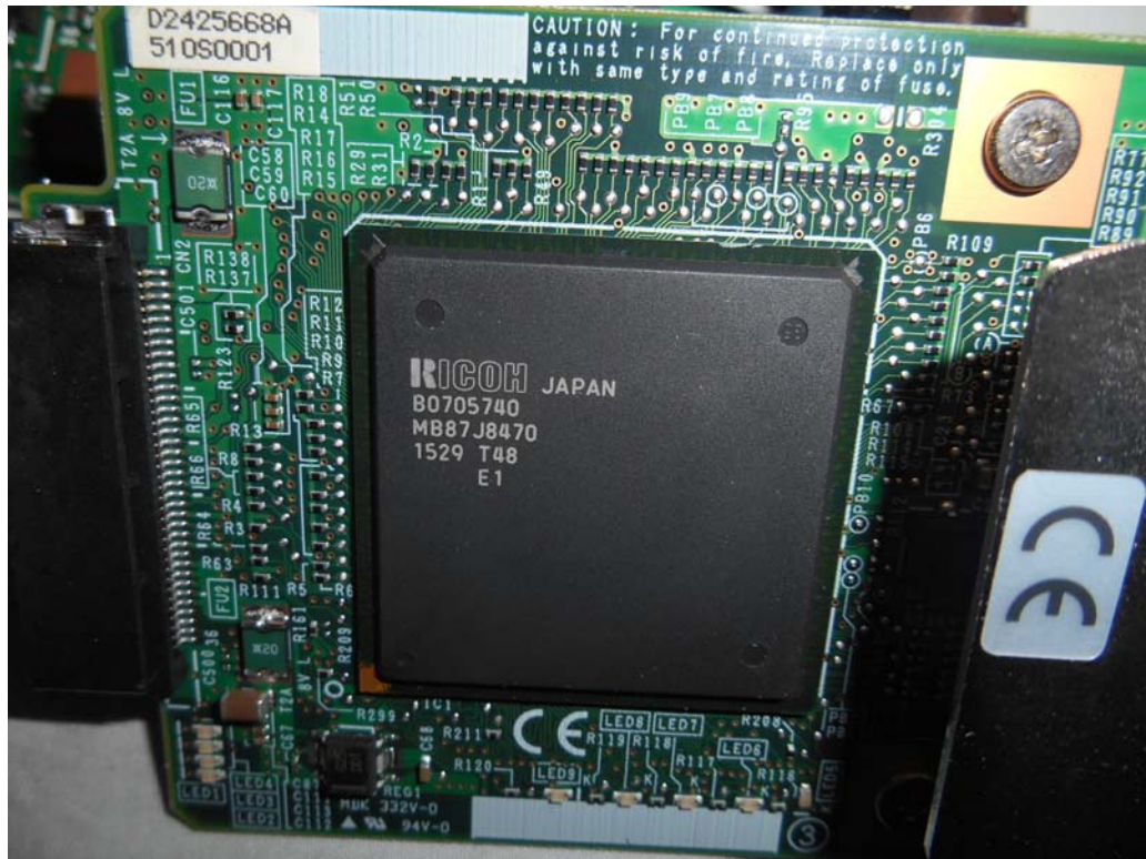
FIGURE 98 PRINTER (M/N: SP C342DN SP C340DN ) CHIP AND CRYSTAL ON IEEE1284 BOARD
