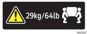
The machine weighs approximately 29 kg (64 lb.). When moving the machine, use the inset grips on both sides, and lift slowly in pairs.
