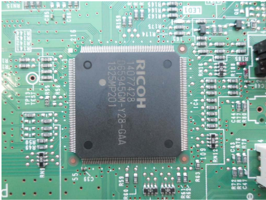
FIGURE 7 PRINTER (M/N: SP C252DN) CHIP #1 ON MAIN BOARD
