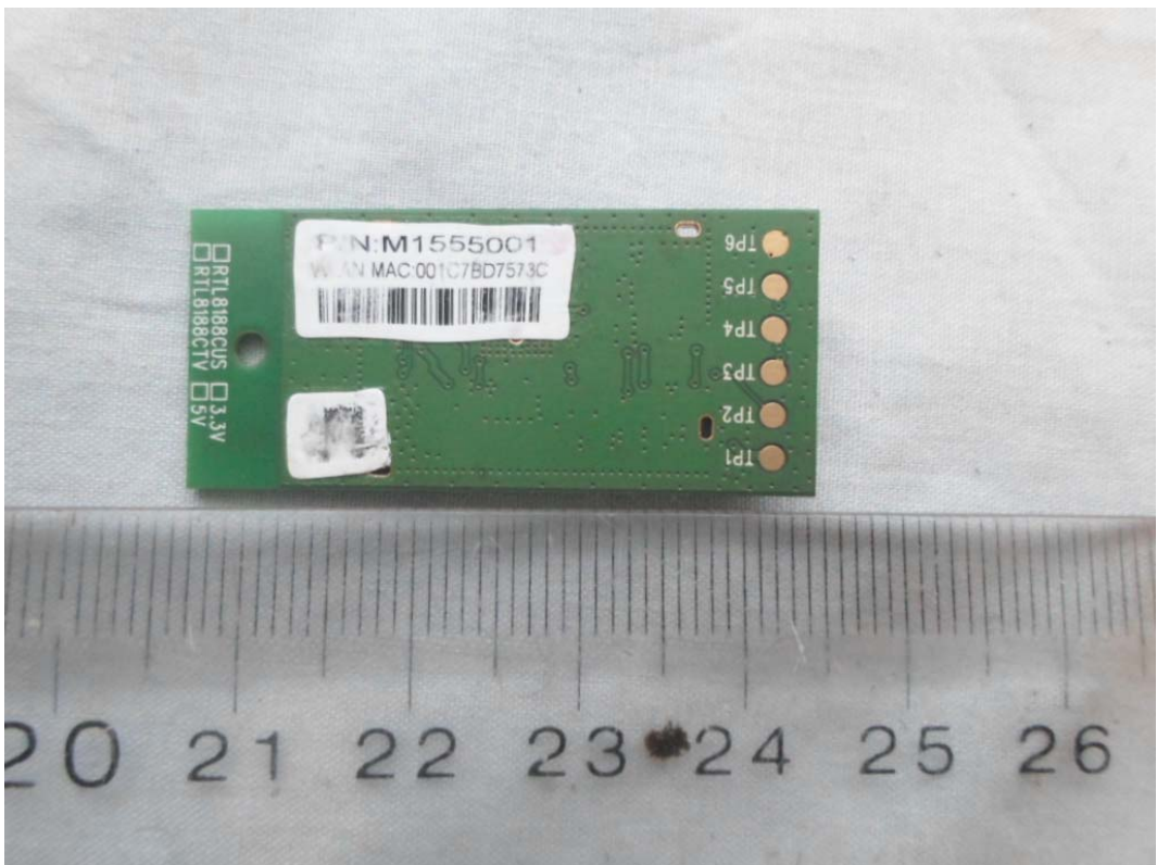
FIGURE 21 PRINTER (M/N: SP C252DN) WIFI BOARD (SOLDERED SIDE)
