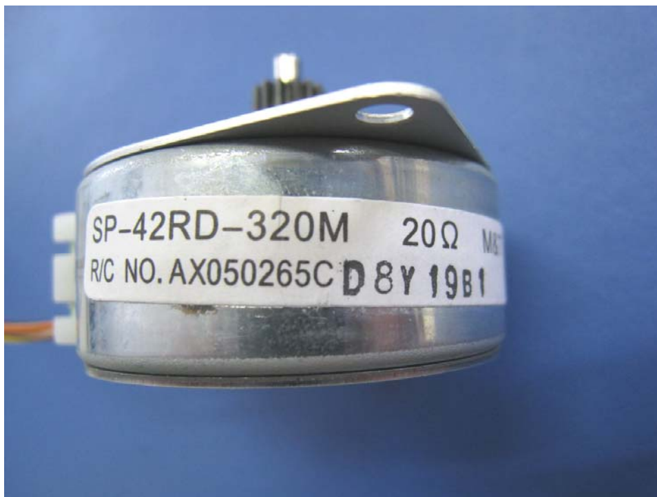
Photo of Duplex stepping motor (with S/N)
