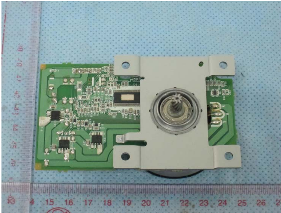
Photo of DC main motor (back)
