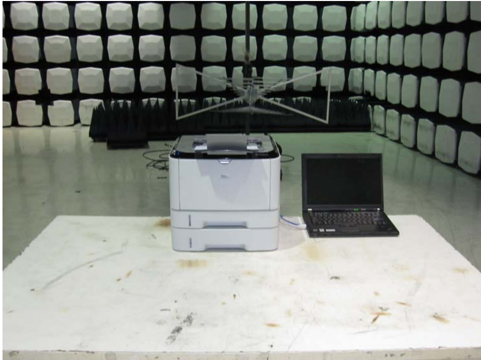
Radiated emission test setup
