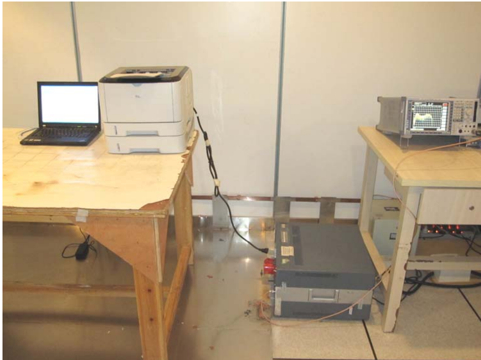
Conducted disturbance test setup
