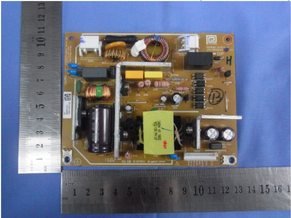
Figure 10 Internal View (Power Board/ Front View)
