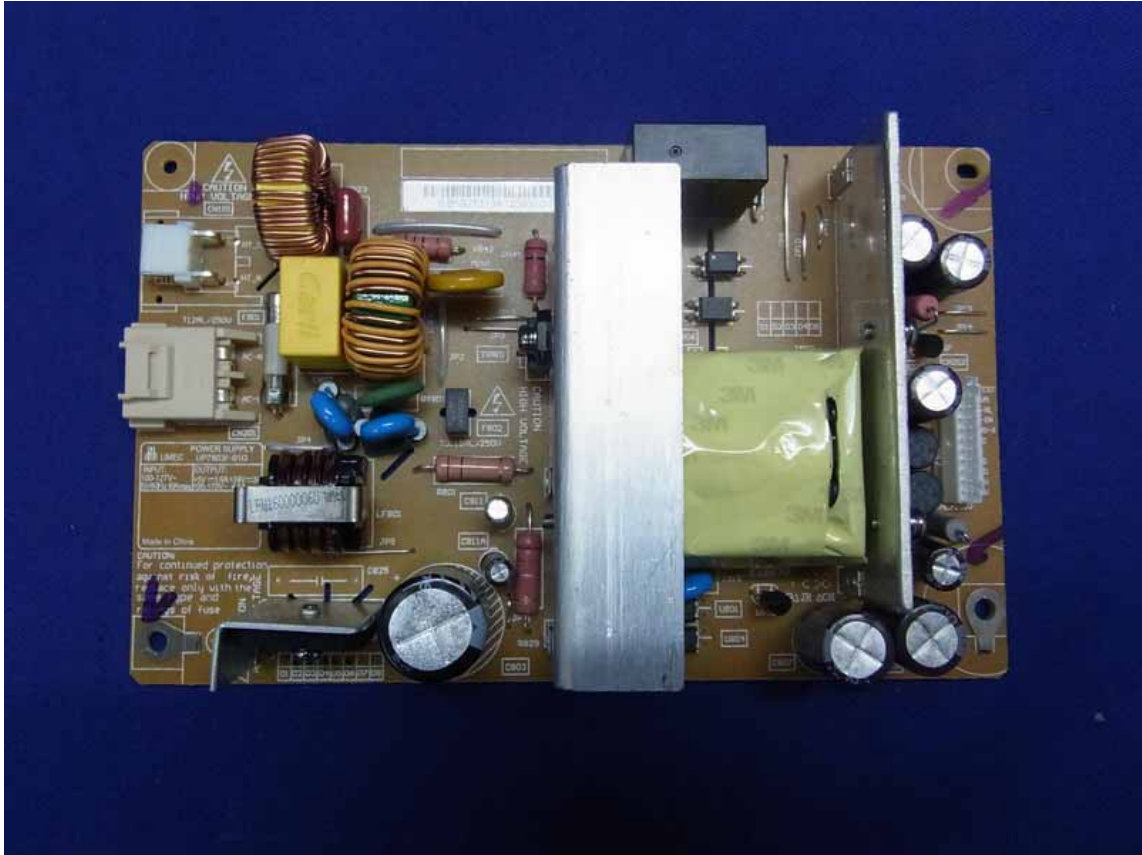
Figure 11 Frontside of the Power Board
