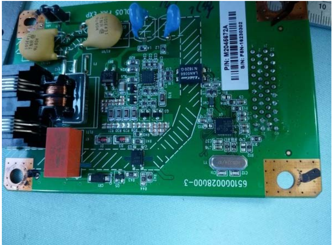
FIGURE 24 PRINTER (M/N: SP C262SFNW) CHIP AND CRYSTAL ON POTS BOARD
