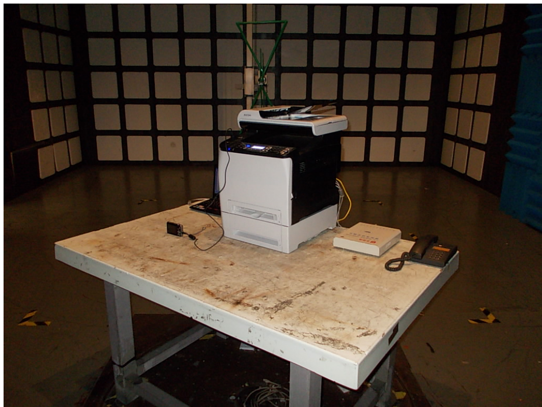
SETUP WITH MAXIMUM DETECTED EMISSION AT VERTICAL POLARIZATION (TEST MODE: WIFI PRINT)
