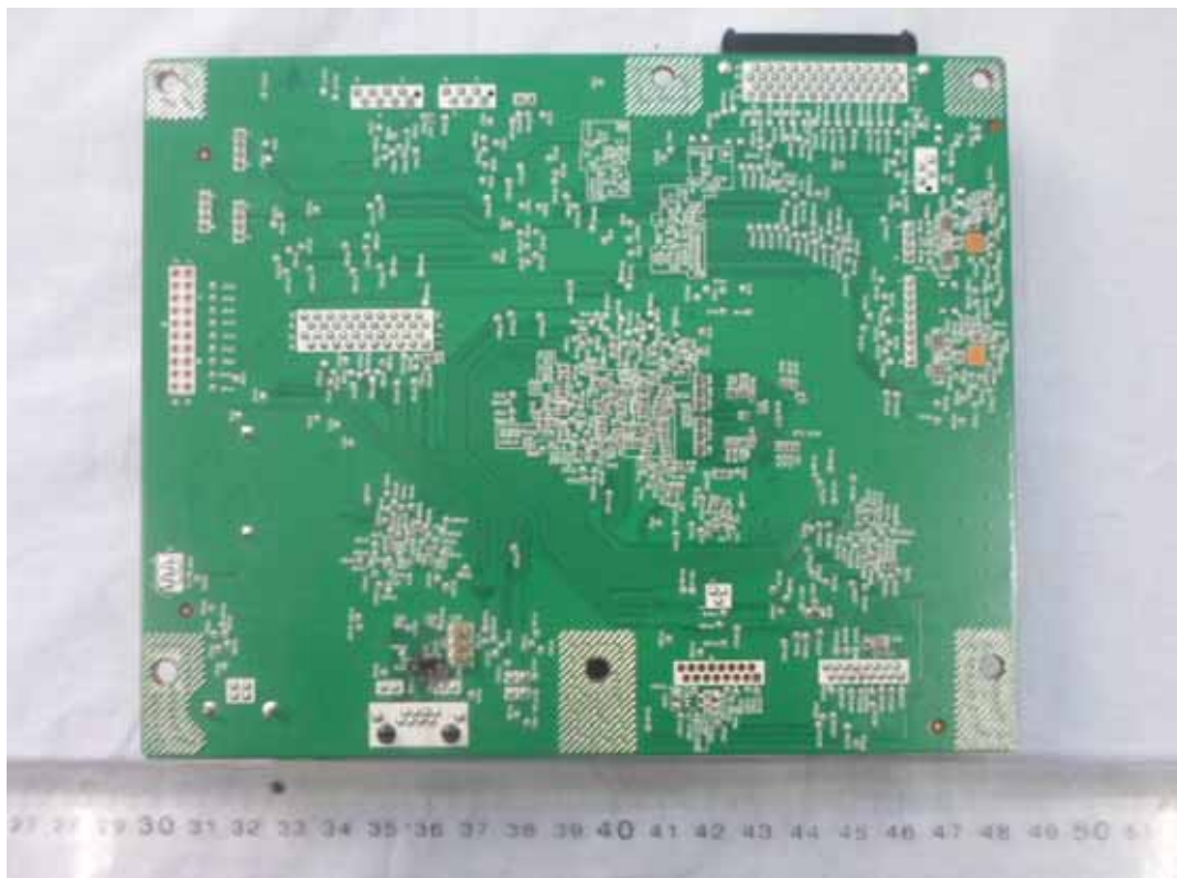
FIGURE 7 PRINTER (M/N: SP C252SF) SIGNAL BOARD (SOLDERED SIDE)
