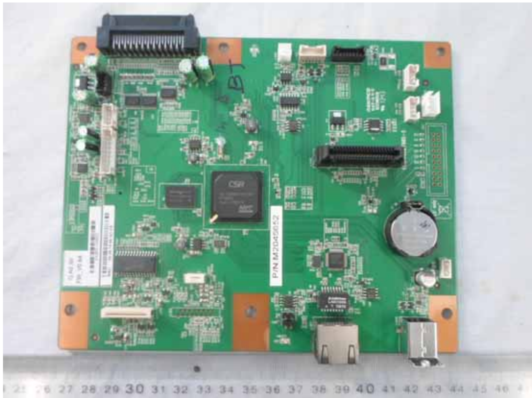
FIGURE 6 PRINTER (M/N: SP C252SF) SIGNAL BOARD (COMPONENT SIDE)
