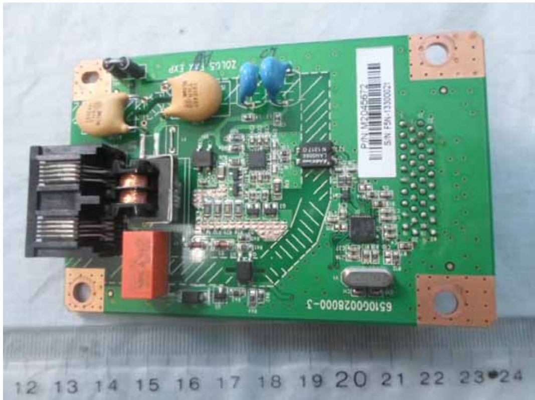
FIGURE 4 PRINTER (M/N: SP C252SF) POTS BOARD (COMPONENT SIDE)
