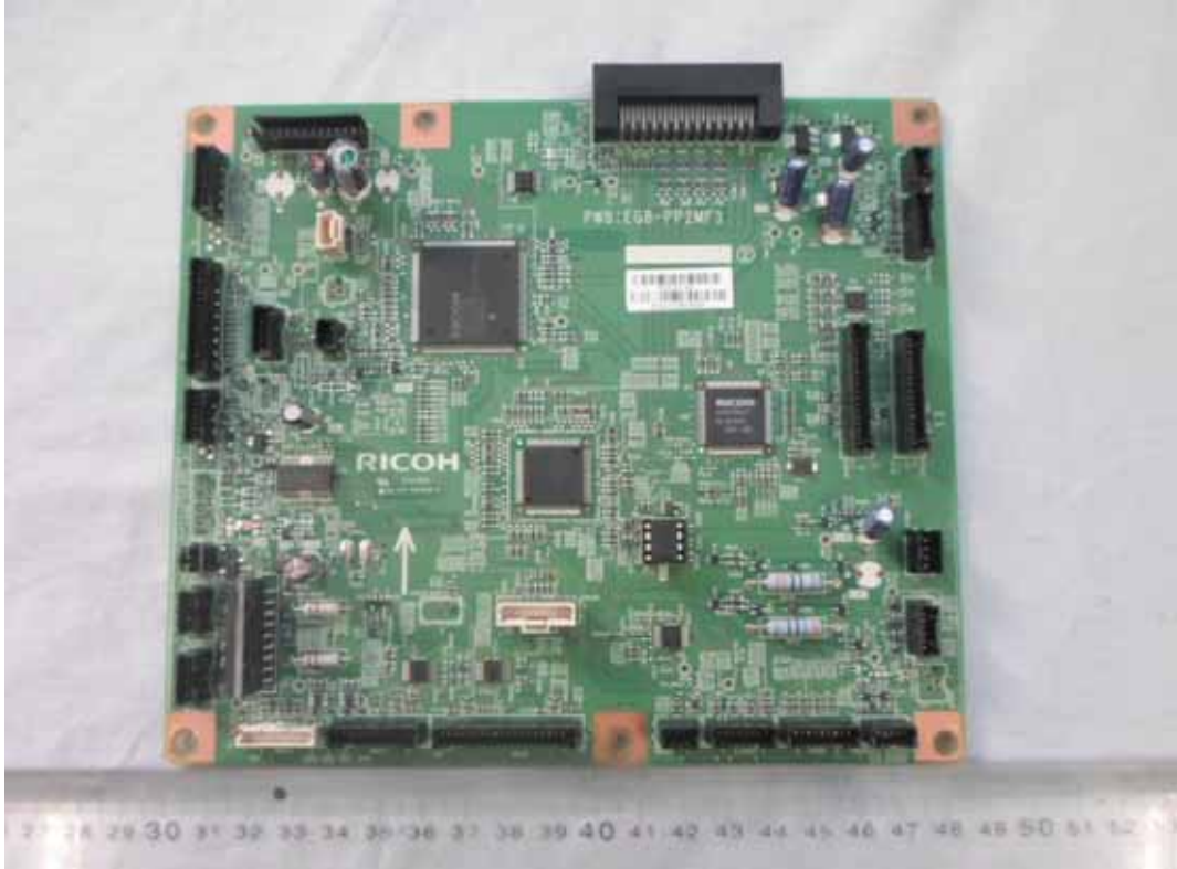
FIGURE 9 PRINTER (M/N: SP C252SF) MAIN BOARD (COMPONENT SIDE)
