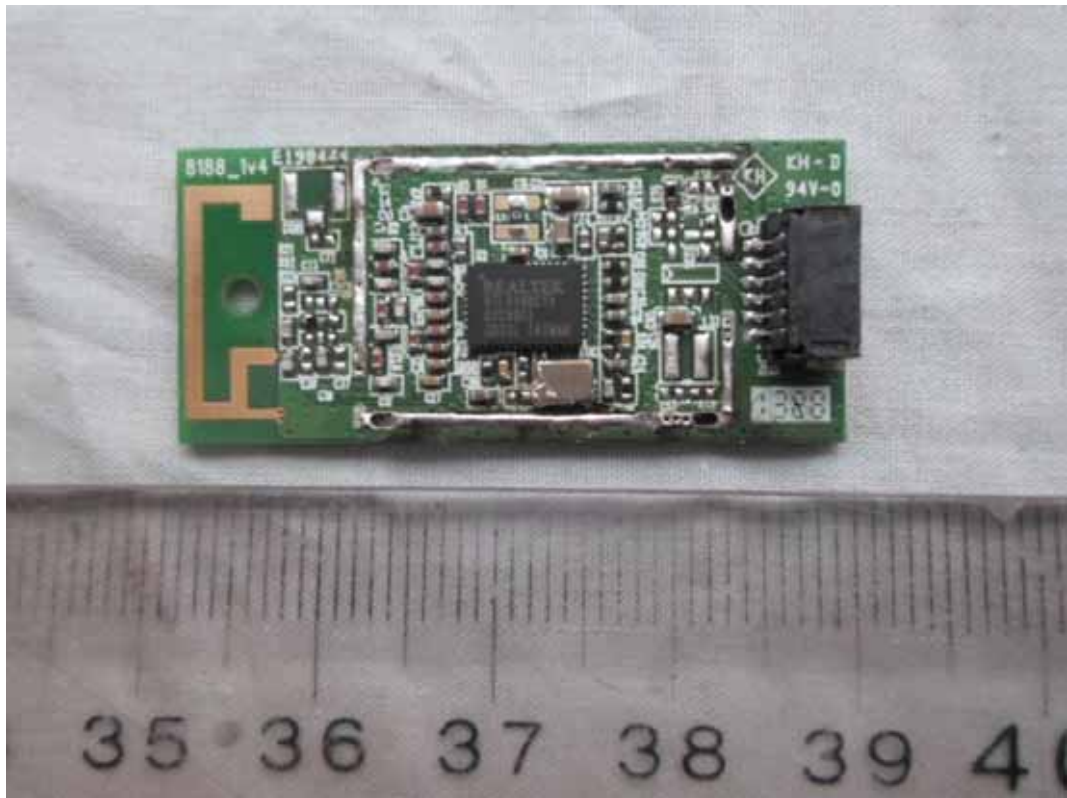
FIGURE 24 PRINTER (M/N: SP C252SF) WIFI BOARD (COMPONENT SIDE)
