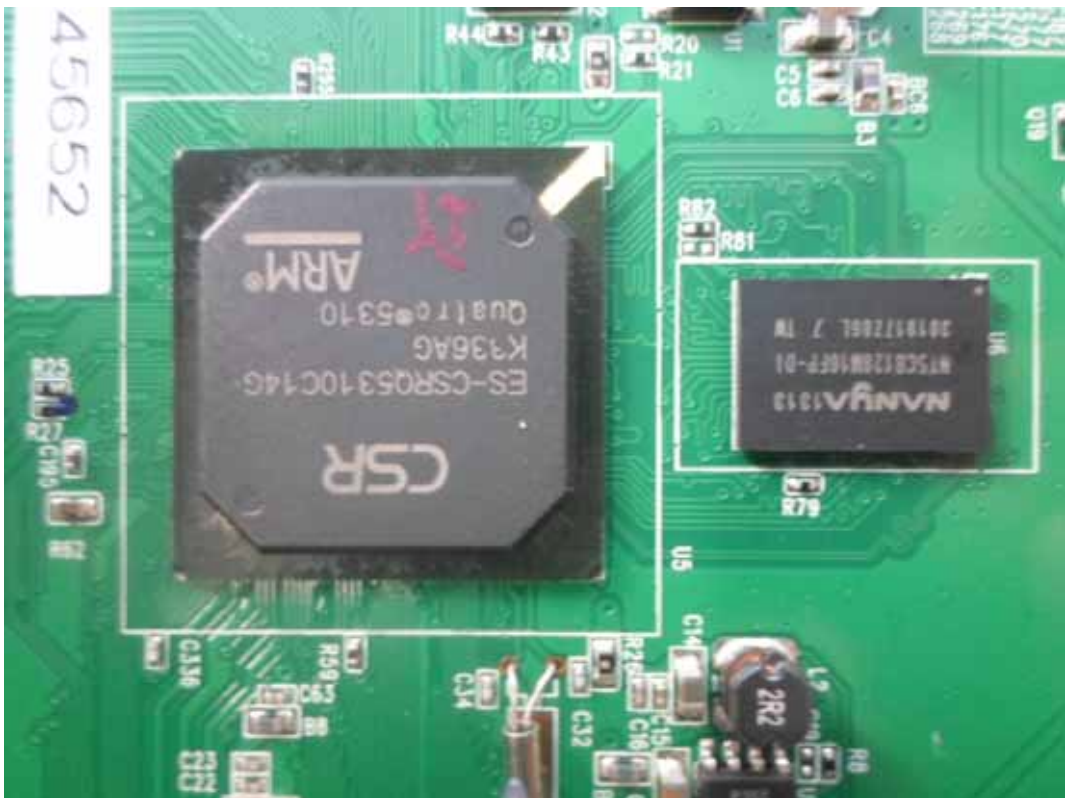
FIGURE 8 PRINTER (M/N: SP C252SF) CHIP ON SIGNAL BOARD
