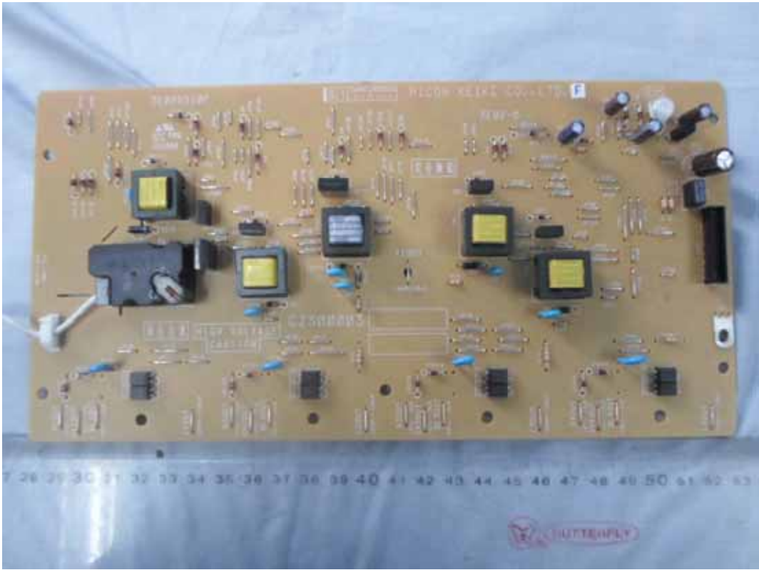
FIGURE 16 PRINTER (M/N: SP C252SF) POWER BOARD #2 (COMPONENT SIDE)
