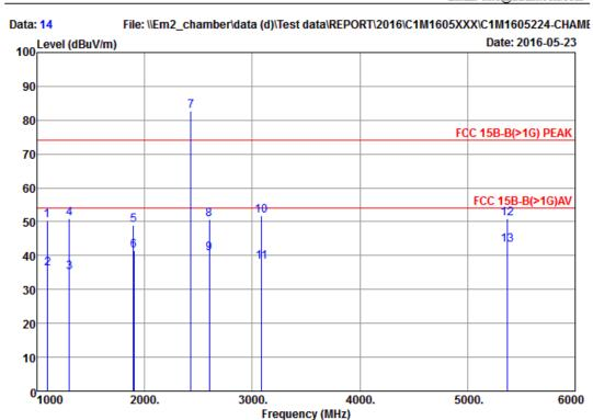
EUT : SP 325SFNW Power Rating : 120Vac/60Hz Test Mode : FAX-RX
