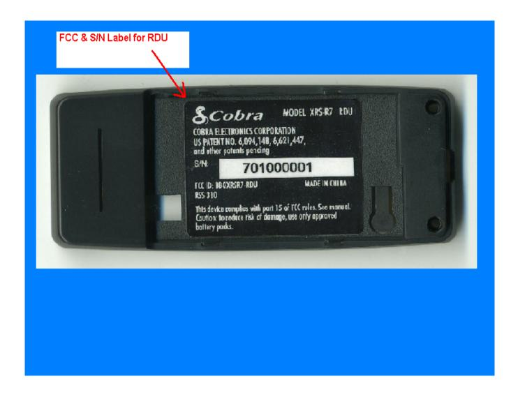
The label will be applied to the RDU behind the battery in the battery compartment.
