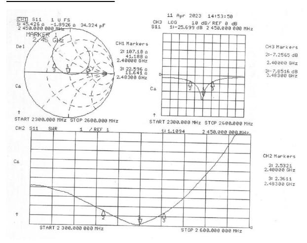
Passive Matching Values: Series 6pF – Series 4.3nH – Shunt 1.5pF – Antenna
