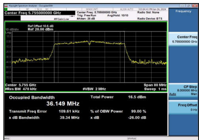
U-NII-3 99% & 26dB Bandwidth-802.11ac(80MHz) ,5775MHz,Ant1
