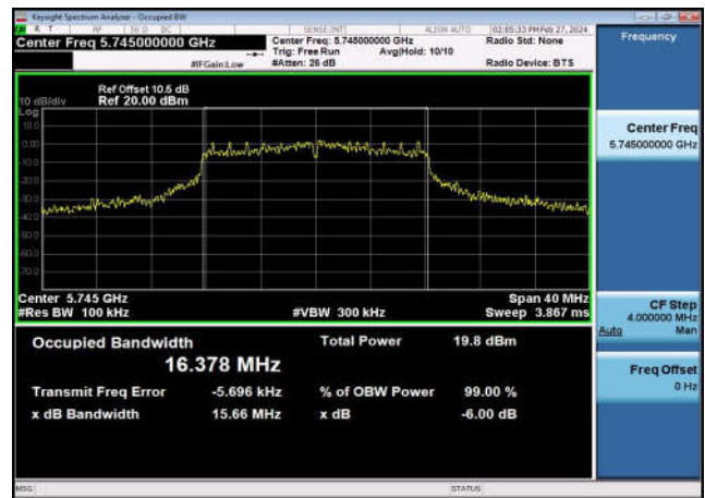
U-NII-3 6dB Bandwidth-802.11a(20MHz) ,5745MHz,Ant1
