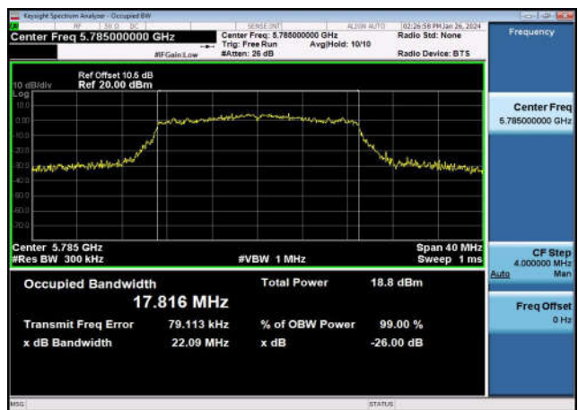
U-NII-3 99% & 26dB Bandwidth-802.11n(40MHz),5755MHz,Ant1
