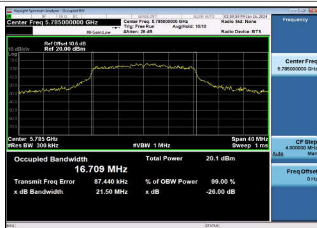
U-NII-3 99% & 26dB Bandwidth-802.11ac(20MHz) ,5745MHz,Ant1
