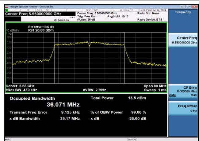
U-NII-2c 99% & 26dB Bandwidth-802.11ac(40MHz) ,5550MHz,Ant1
