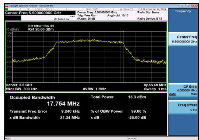
U-NII-2c 99% & 26dB Bandwidth-802.11ac(20MHz) ,5700MHz,Ant1
