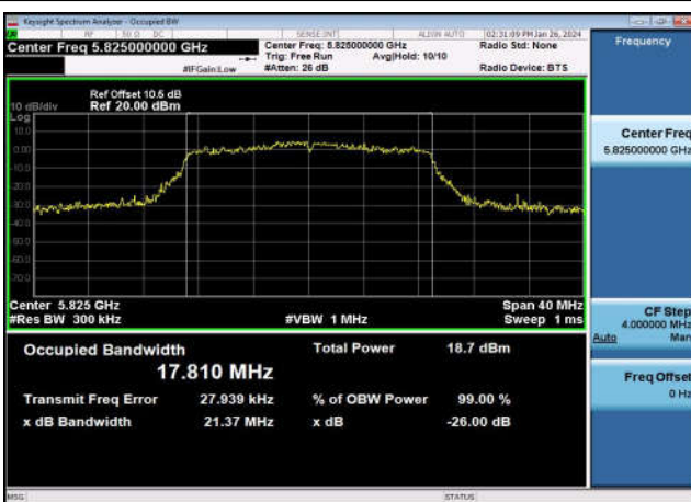
U-NII-3 99% & 26dB Bandwidth-802.11n(20MHz),5825MHz,Ant1
