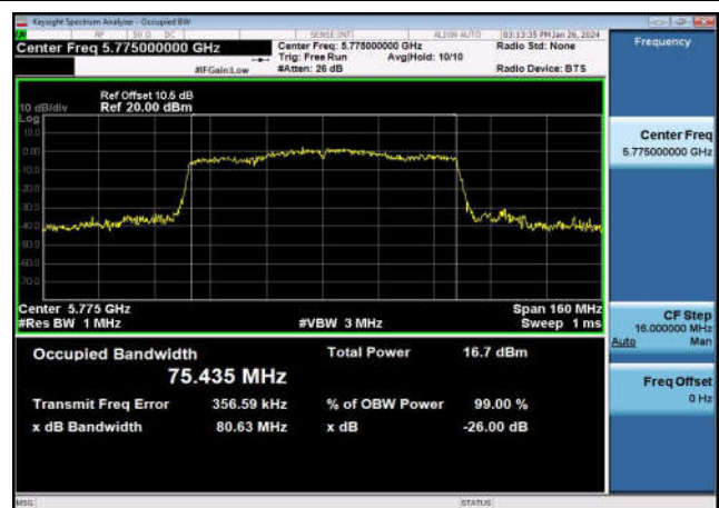
U-NII-3 99% & 26dB Bandwidth-802.11ac(80MHz) ,5775MHz,Ant1
