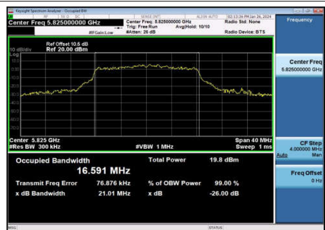
U-NII-3 99% & 26dB Bandwidth-802.11ac(20MHz) ,5785MHz,Ant1
