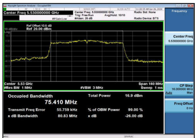
U-NII-3 99% & 26dB Bandwidth-802.11n(20MHz),5785MHz,Ant1
