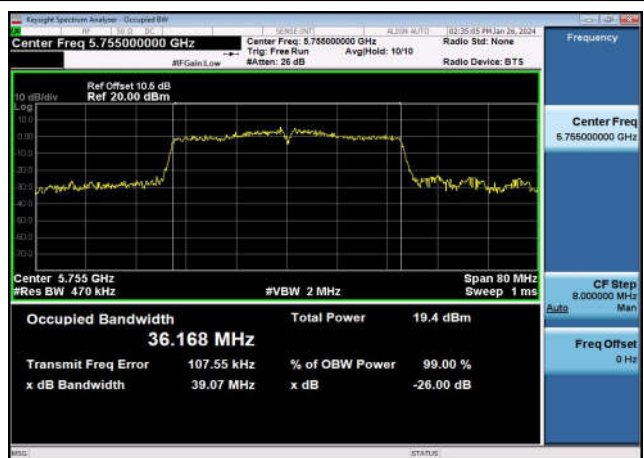
U-NII-3 99% & 26dB Bandwidth-802.11n(40MHz),5755MHz,Ant1
