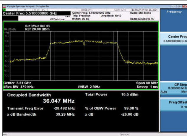
U-NII-2c 99% & 26dB Bandwidth-802.11ac(40MHz) ,5510MHz,Ant1
