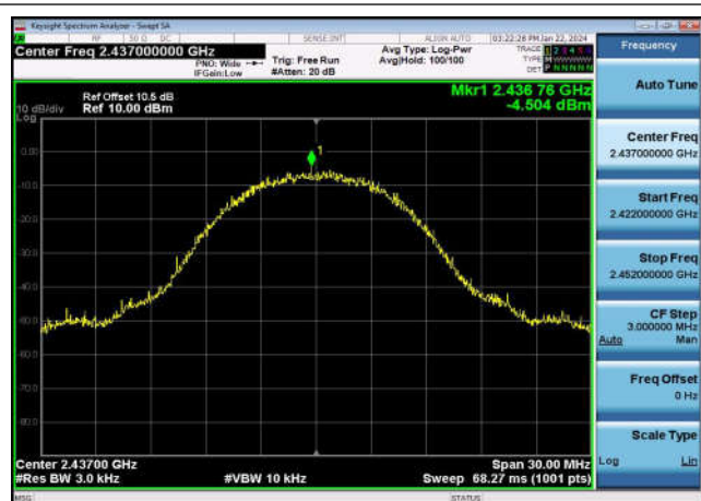
Power spectral density-802.11g ,2412MHz,Ant0
