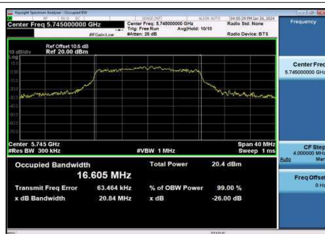
U-NII-3 99% & 26dB Bandwidth-802.11a(20MHz) ,5825MHz,Ant1
