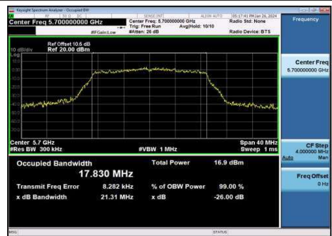
U-NII-2c 99% & 26dB Bandwidth-802.11ac(40MHz) ,5550MHz,Ant1
