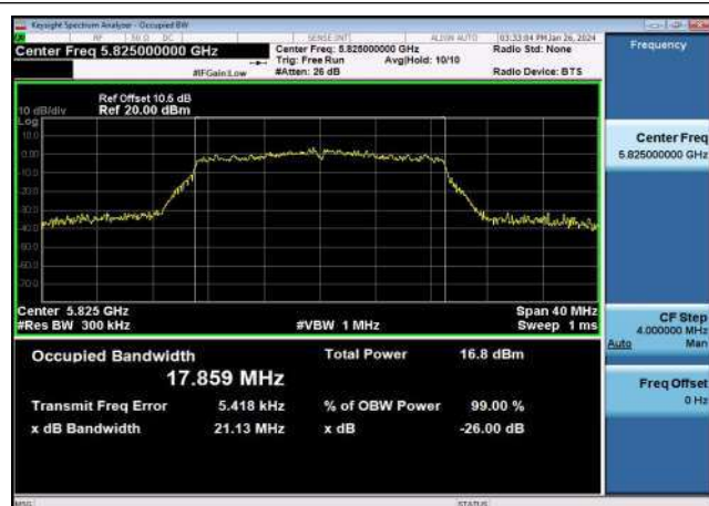
U-NII-3 99% & 26dB Bandwidth-802.11ac(40MHz) ,5795MHz,Ant1
