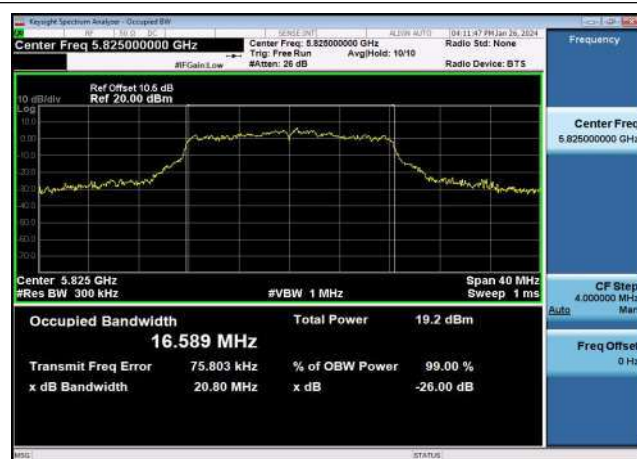
U-NII-3 99% & 26dB Bandwidth-802.11ac(20MHz) ,5785MHz,Ant1
