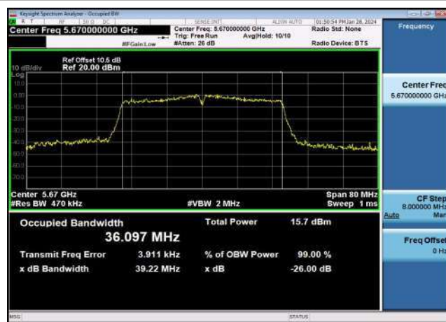
U-NII-3 99% &amp; 26dB Bandwidth-802.11n(20MHz),5745MHz,Ant1
