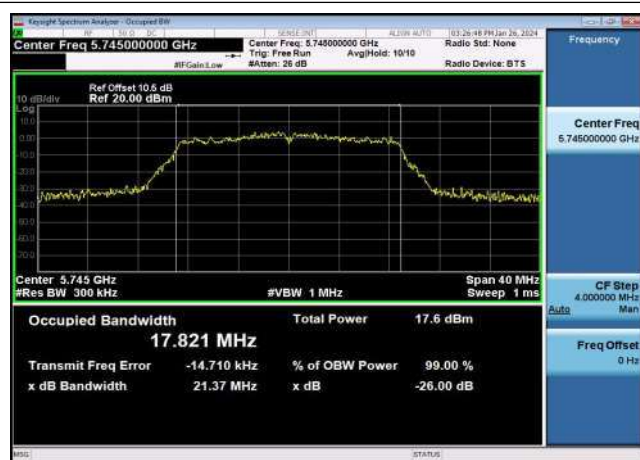
U-NII-3 99% & 26dB Bandwidth-802.11ac(20MHz) ,5745MHz,Ant1
