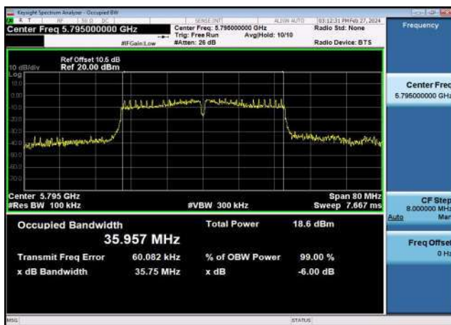
U-NII-3 6dB Bandwidth-802.11n(40MHz) ,5795MHz,Ant1
