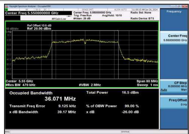
U-NII-2c 99% & 26dB Bandwidth-802.11ac(40MHz) ,5550MHz,Ant1
