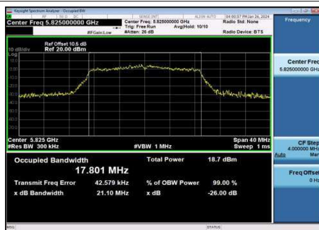
U-NII-3 99% &amp; 26dB Bandwidth-802.11n(20MHz),5825MHz,Ant1
