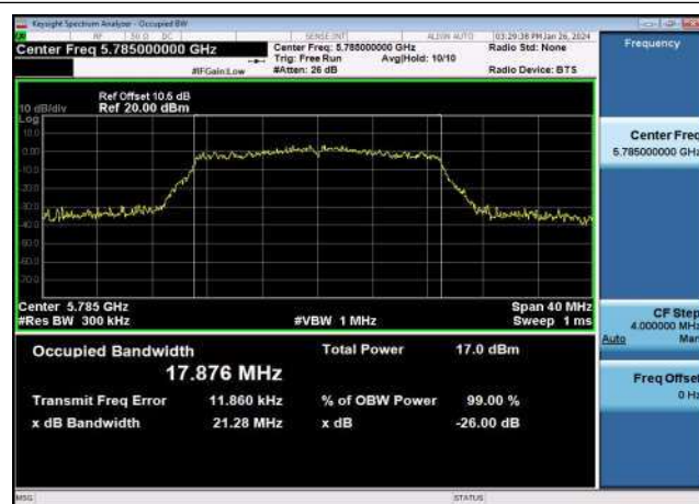
U-NII-3 99% & 26dB Bandwidth-802.11ac(20MHz) ,5785MHz,Ant1
