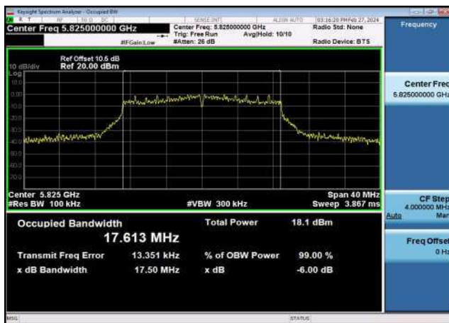
U-NII-3 6dB Bandwidth-802.11n(40MHz) ,5795MHz,Ant1
