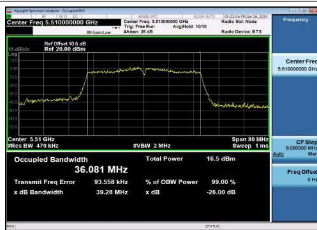
U-NII-2c 99% & 26dB Bandwidth-802.11ac(40MHz) ,5510MHz,Ant1
