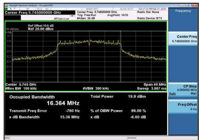
U-NII-3 6dB Bandwidth-802.11a(20MHz) ,5745MHz,Ant1
