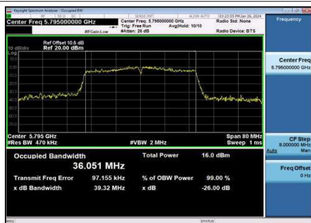
U-NII-3 99% & 26dB Bandwidth-802.11ac(40MHz) ,5795MHz,Ant1
