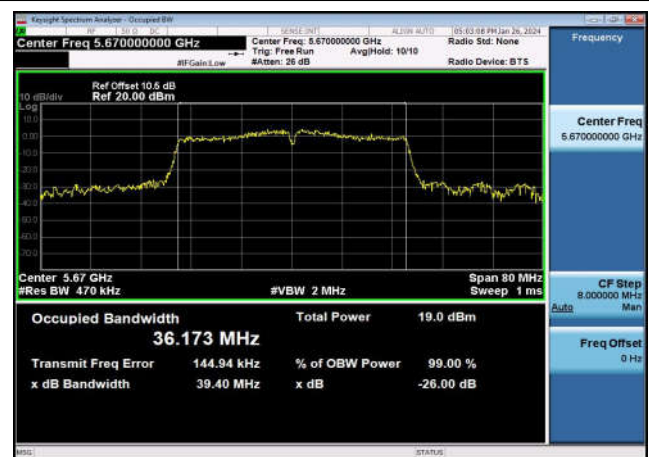
U-NII-2c 99% & 26dB Bandwidth-802.11a(20MHz) ,5580MHz,Ant1
