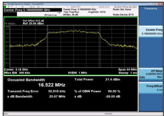
U-NII-1 99% & 26dB Bandwidth-802.11a(20MHz) ,5180MHz,Ant1
