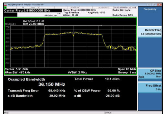
U-NII-2c 99% & 26dB Bandwidth-802.11n(40MHz) ,5670MHz,Ant1
