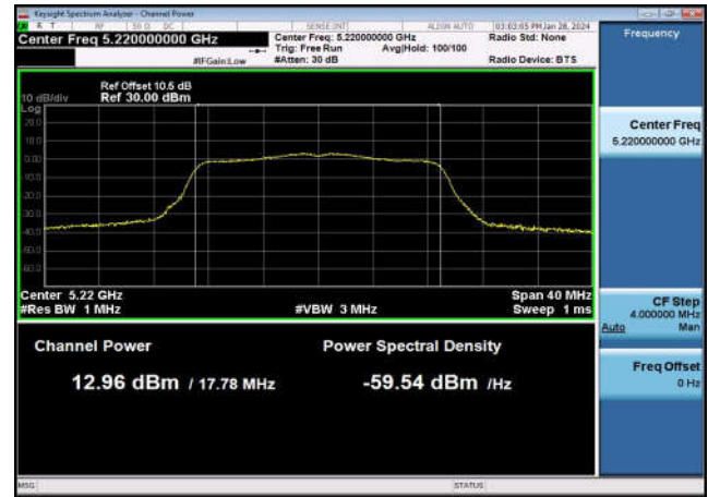
U-NII-1 Output Power-802.11n(40MHz) ,5190MHz,Ant1
