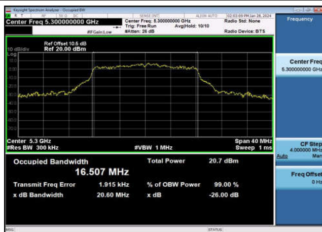
U-NII-2a 99% & 26dB Bandwidth-802.11ac(20MHz) ,5260MHz,Ant1
