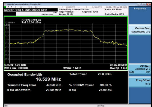
U-NII-2a 99% & 26dB Bandwidth-802.11a(20MHz) ,5320MHz,Ant1
