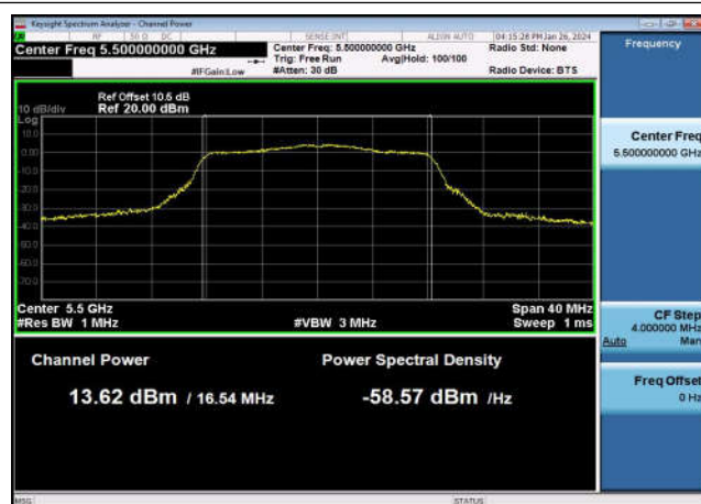
U-NII-2c Output Power-802.11a(20MHz) ,5500MHz,Ant1
