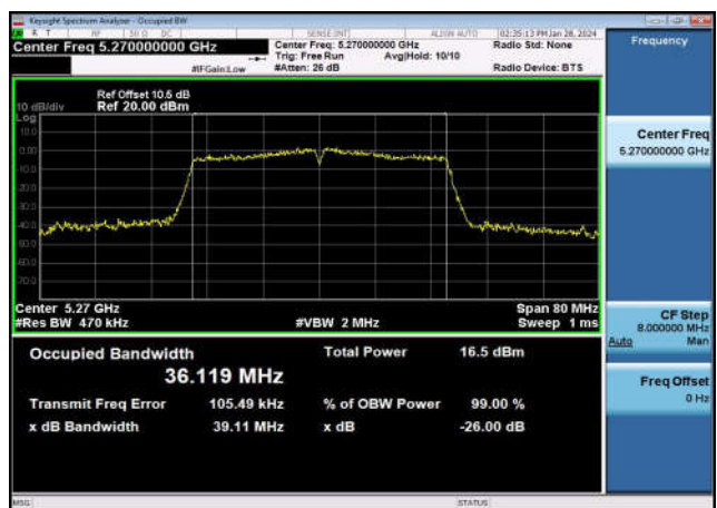
U-NII-2a 99% & 26dB Bandwidth-802.11ac(80MHz),5290MHz,Ant1
