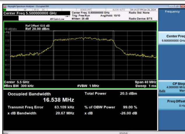
U-NII-2c 99% & 26dB Bandwidth-802.11a(20MHz) ,5500MHz,Ant1
