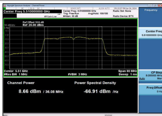
U-NII-2c Output Power-802.11ac(40MHz) ,5510MHz,Ant1
