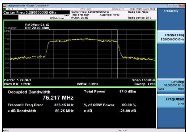
U-NII-2c 99% & 26dB Bandwidth-802.11n(20MHz),5580MHz,Ant1
