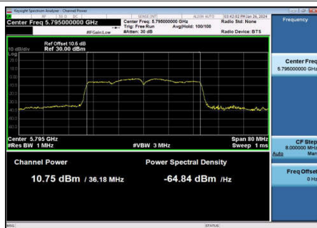
U-NII-3 Output Power-802.11a(20MHz) ,5785MHz,Ant1
