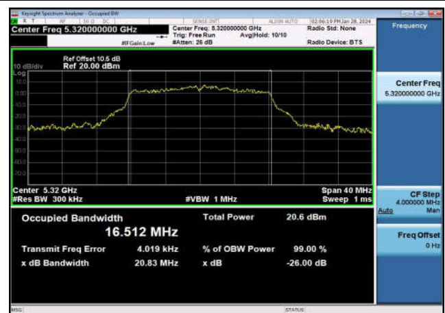
U-NII-2a 99% & 26dB Bandwidth-802.11ac(20MHz) ,5300MHz,Ant1
