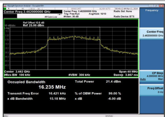
6dB Bandwidth-802.11g,2462MHz,Ant0
