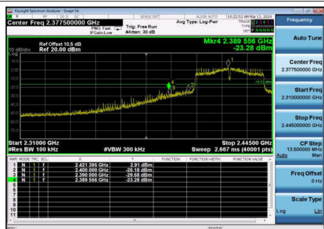
,Plot 2,Band Edge-802.11n(40MHz ,2452MHz,Ant0
