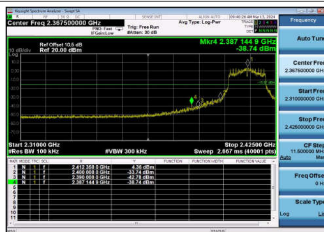
,Plot 2,Band Edge-802.11g,2462MHz ,Ant0
