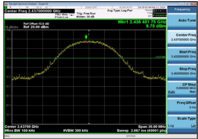
,Plot 2,Band Edge-802.11b,2412MHz ,Ant0
