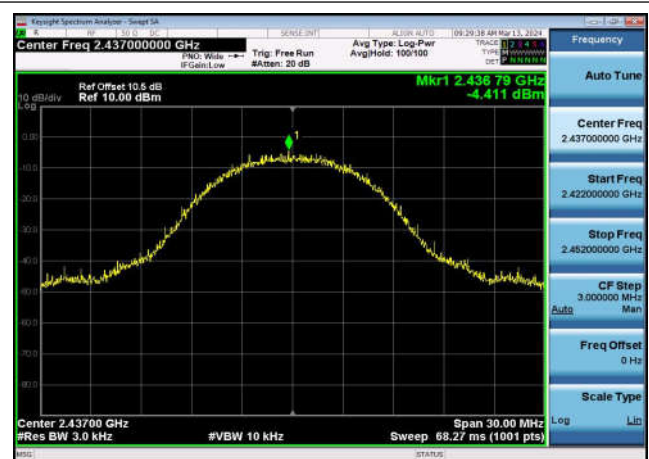
Power spectral density-802.11g ,2412MHz,Ant0
