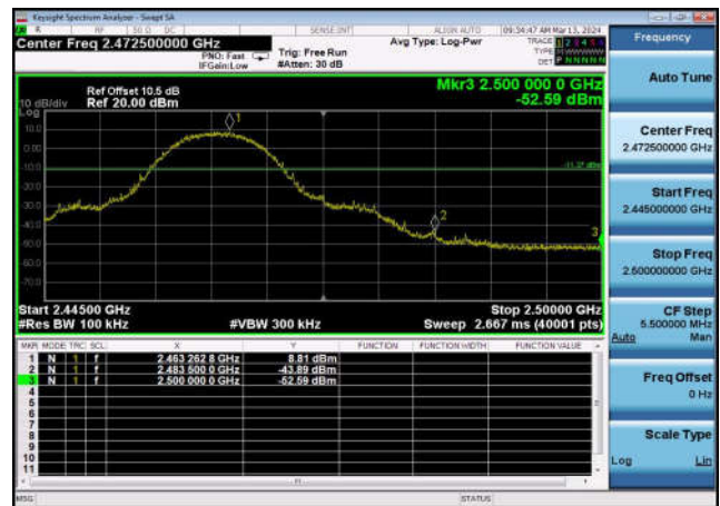
,Plot 2,Band Edge-802.11b,2462MHz ,Ant0
