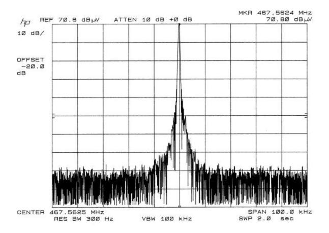
APPLICANT: COBRA ELECTRONICS CORPORATION FCC ID: BBOPR945 REPORT #: C\COBRA\1173AUT2\1173AUT2TestReport.doc Page 12 of 20 Spurious emissions at antenna terminals(conducted): The following data shows the level of conducted spurious responses at the antenna terminal. The test procedure used was TIA/EIA 603 S2.2.13 with the exception that the emissions were recorded in dBc. The spectrum was scanned from 0.4 to at least the 10th harmonic of the fundamental.
