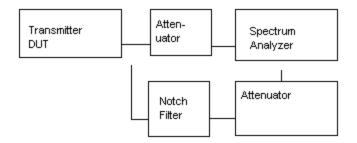
Method of Measuring Conducted Spurious Emissions
